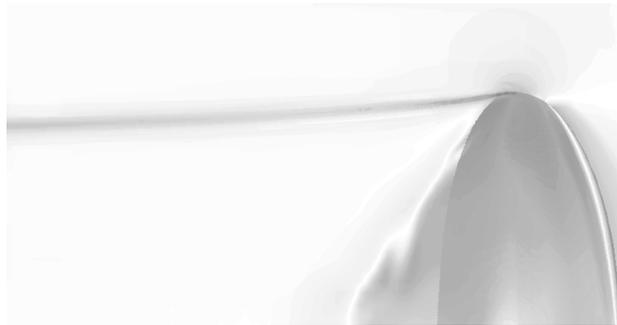
**Figure 8:** Contour plot of constant pressure visualizing the shape of the vortex stretching downstream from the hydrofoil tip. The flow is from right to left. The low pressure regions close to the trailing edge is caused by shedding from the suction side of the foil.
