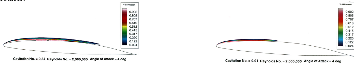
Fig. 9. Cavitation bubbles indicated by void fraction contours on the NACA 66 modified hydrofoil at cavitation numbers of (a) 0.91 and (b) 0.84.
