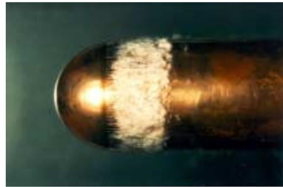
b) developed cavitation at  $\sigma = 0.80$  und  $V_\infty = 14,0$  m/s
