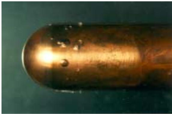
a) beginning cavitation at  $\sigma = 0.80$  und  $V_\infty = 8,0$  m/s
