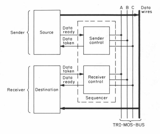
Figure 4: Schematic diagram of a bus participant. The source and destination will drive and sense the data wires respectively. The sequencer converts between TRIMOSBUS sequencing signals and conventional two-wire handshaking signals.
