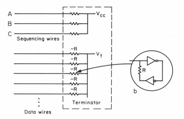
Figure 1: The TRIMOSBUS uses two sorts of wires. Three sequencing wires are terminated to Vcc to permit wired-or operation. An arbitrary number of data wires is provided, each terminated with a negative resistance to the inverter threshold voltage Vt. This negative resistance termination allows the wires to be used reliably as storage nodes. Inset: one implementation for the negative resistance termination.
