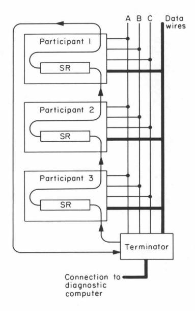
Figure 7: A serial communication line is used to read and write the state of the bus participants for debugging.
