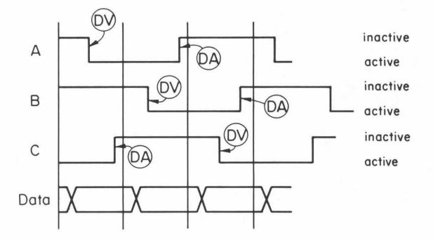
Figure 3: Each bus cycle requires three transitions. The first drives data wires to the correct state. The second indicates data validity (DV) by clamping a sequencing wire. The third indicates data acceptance (DA) by all receivers when a sequencing wire becomes inactive.
