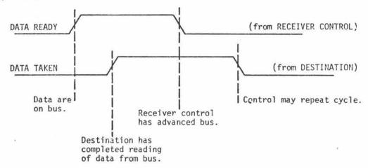
Figure 6: Two-wire handshaking signals used by the sequencer. Two variations of the sender control are shown. The first allows the data wires to provide a single level of buffering between the sender and the receivers.
