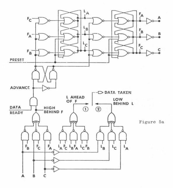
Figure 5: Logic diagram for sender (5a) and receiver (5b) of experimental TRIMOSBUS control for use as shown in Figures 4 and 6. The DATA READY signal in the sender circuit may be derived from source (1) or source (2), corresponding to the signaling interpretations shown in Figures 6a and 6b. The receiver circuit can be seen to be very similar to that for the sender.
